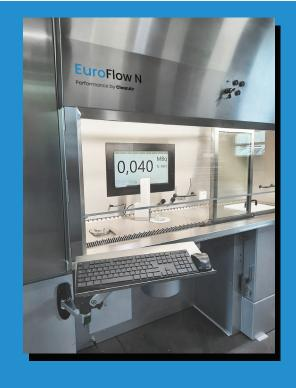
The EuroFlow N is a range of high-quality Class II biological safety cabinets. The EF-N unit is configured with features such as lead shielding for the interior, generator chamber, waste safe, and dose calibrator.
